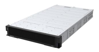
SC6100 is a next-generation 2U rackmount all-flash storage controller for the enterprise. It is powered by two AMD EPYC<sup>™</sup> 9004 series of high-performance microprocessors based on the Zen 4 microarchitecture and supports up to 24 dual-port U.2 PCIe Gen 5 solid state drives (SSDs). The SC6100 delivers extreme performance with high availability for the most demanding enterprise application workloads.
